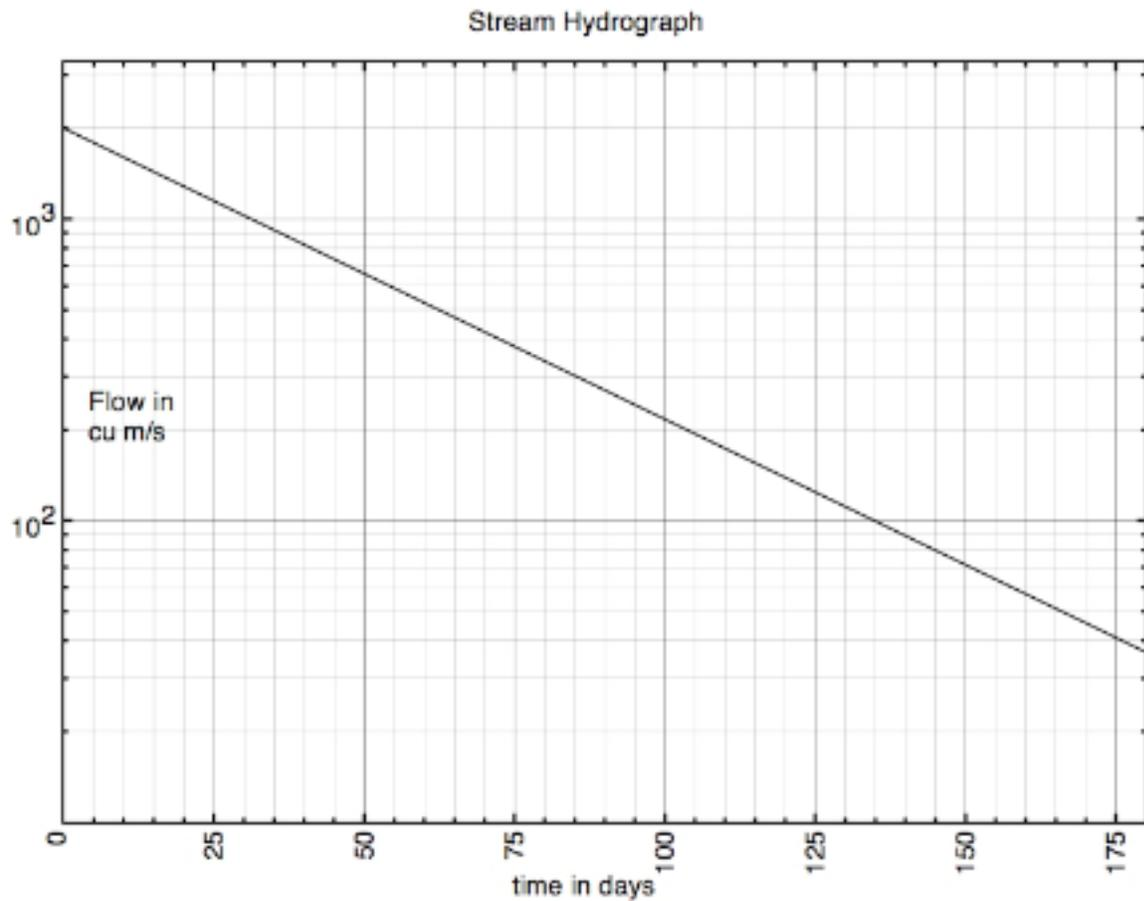
3. Consider the stream hydrograph below. Use the Rorabaugh method to find the total recharge. Recall that the steps are:
