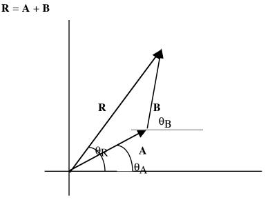
We draw each vector by drawing an arrow to scale with the correct length with the correct angle. Note that the angle is always measured from horizontal. We measure the length of the resultant and the angle, using our scale to compute the magnitude of the resultant vector.
